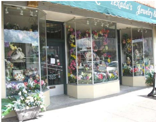
Large display windows and bulkheads beneath them, like these at 606 Main Street, are traditional storefront elements. These bulkheads have applied Carrara glass
